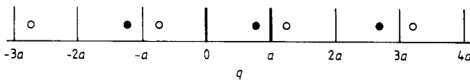
Figure 1. A possible location for the centre of a Gaussian wavepacket and its images for a particle in a one-dimensional box of length a . Bold lines indicate the boundaries of the box. The open and closed circles indicate the relative phase of the wavepackets.
